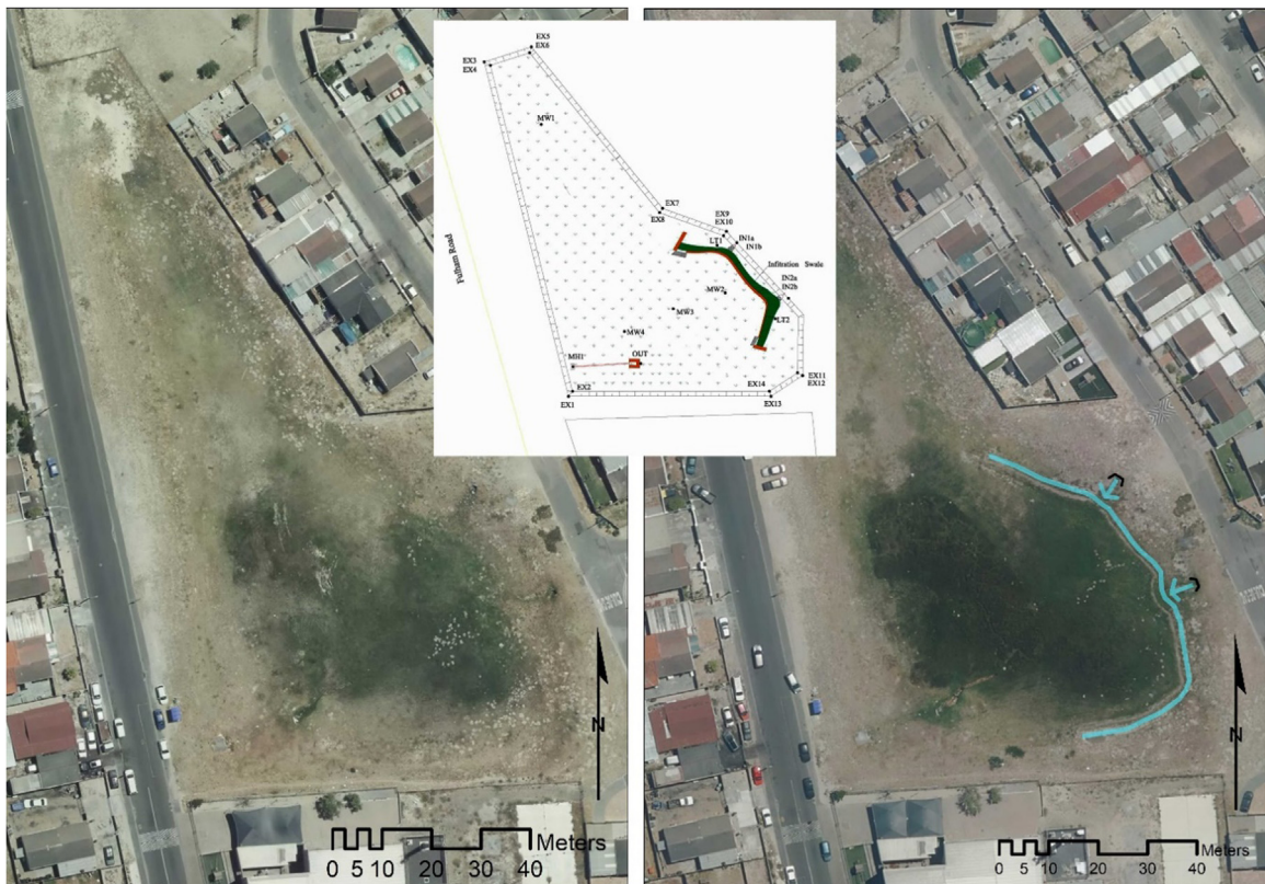
Fig. 2. Aerial image of stormwater pond site before (left) and after (right) construction works, showing outline of completed trench and sandbag wall, positioned to intercept the stormwater inlets based on the technical design (central image) (Sources: CoCT GIS dataset; C. Tanyanyiwa).
