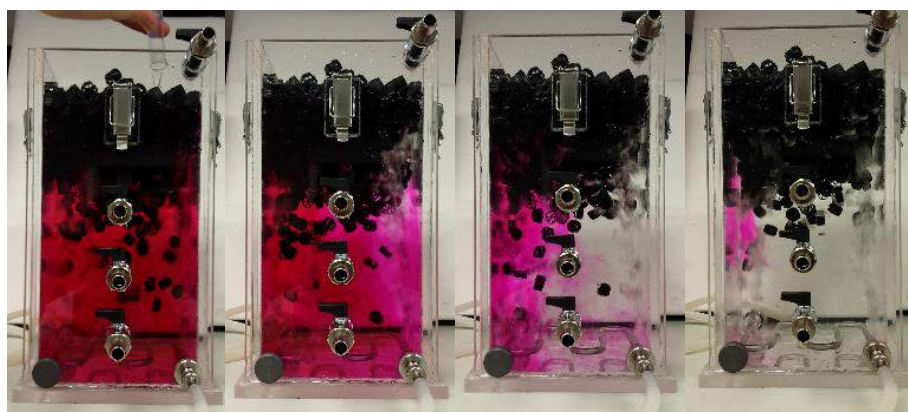
Figure: E-8: Images of phenolphthalein mixing over time for laboratory scale MBBR, with carriers
