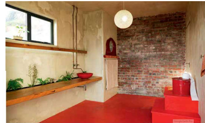
The dry toilet is connected to a drum that can be emptied out once the waste has dried and reduced in volume. Sawdust helps to absorb moisture thus aiding the drying process.
