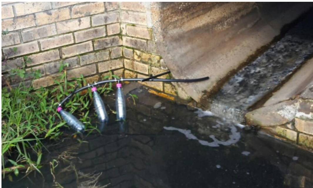
Figure 8.5: Sampling the in and out flow of stormwater by a 'stormwater capture' [155]
