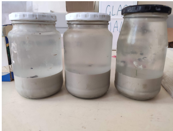
Figure C.5: The samples after sedimentation. The liquid phase was very clear, although the dirt on the jar and the condensation of the fridge doesn't imply this.
