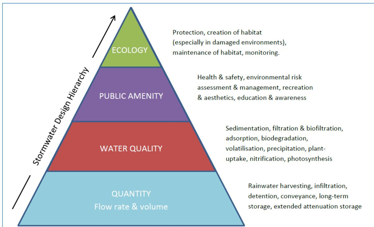
**Figure 5: The SuDS Stormwater Design Hierarchy (after Armitage, et al., 2013)**
