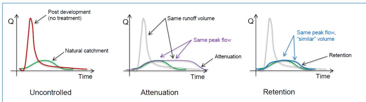
**Figure 1: Demonstrating the principles of attenuation and retention (after Dunsmore, 2017).**
