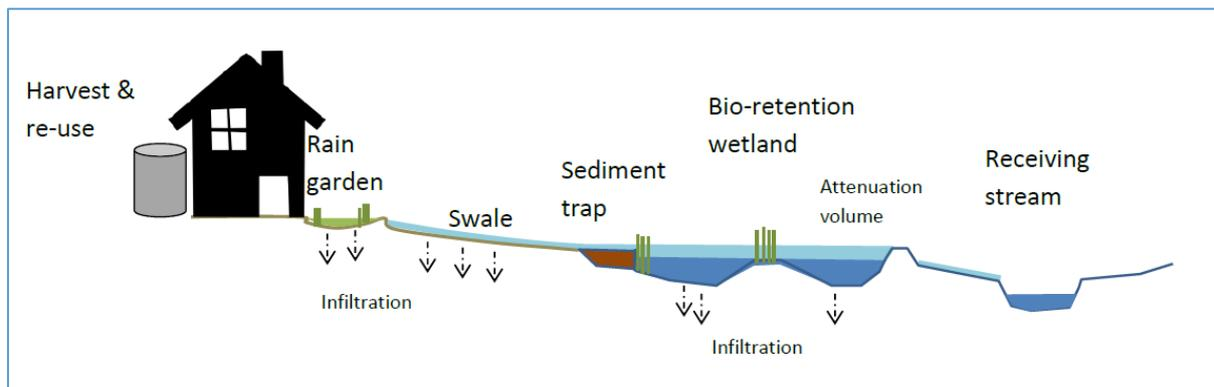
**Figure 3: Example of a treatment train.**
